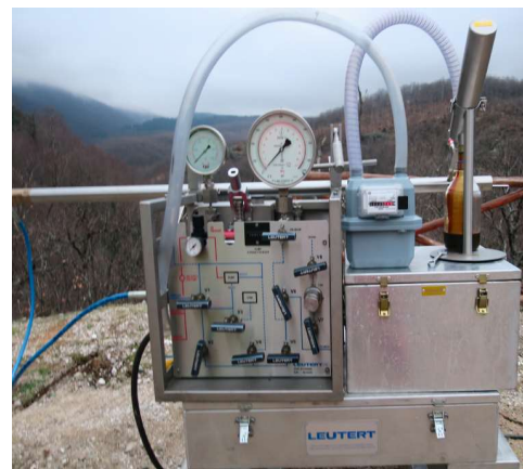
Looking for the 'champagne effect' or liquid gas ratio's
